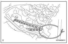
(b) Hold the hexagonal portion of the No. 3 camshaft with a wrench, then loosen the camshaft timing gear set bolt.
