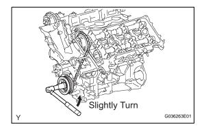
(b) Hold the hexagonal portion of the No. 4 camshaft with a wrench, and remove the camshaft timing gear set bolt.
